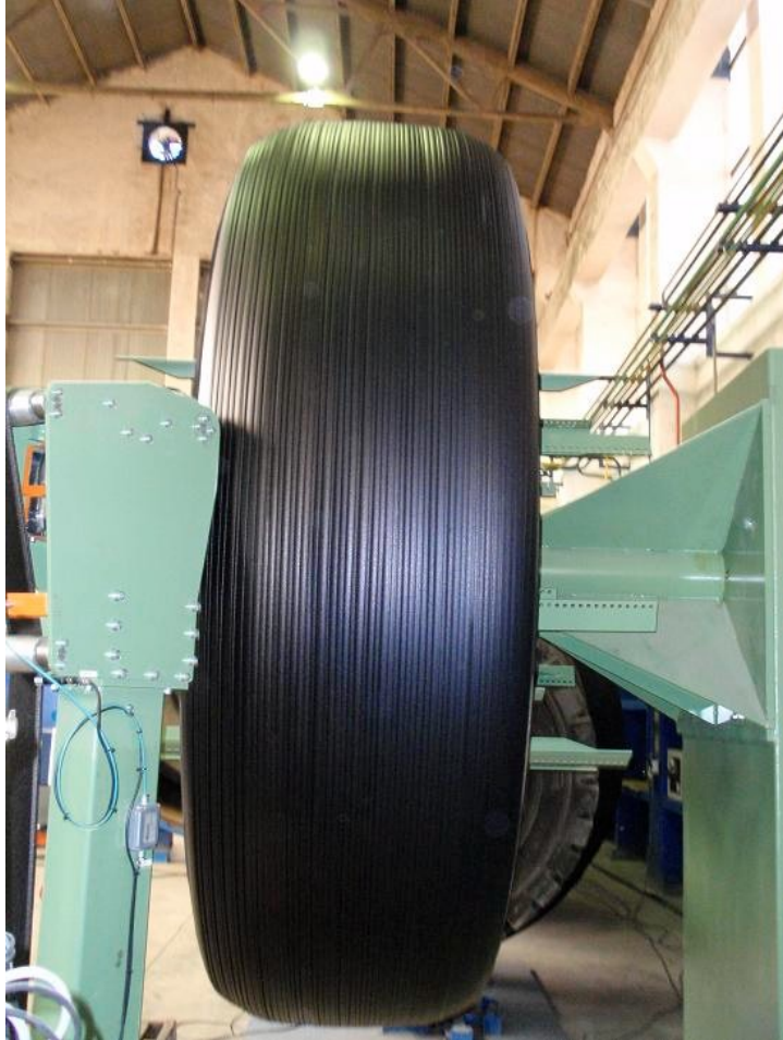
DB ULTRA building station and spin station building a R57 size tyre
