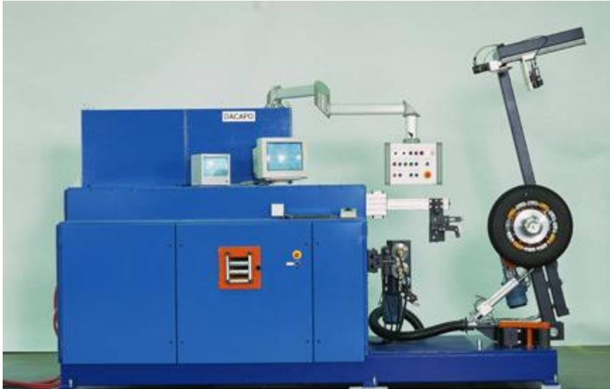
A compact strip wind builder with integral extruder and temperature control system.
